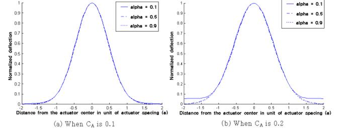
Fig. 3. Normalized influence functions from the derived equation, Eq. (7).
