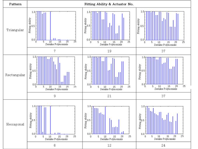
Fig. 7. Fitting ability of the first three layouts of each topology.
