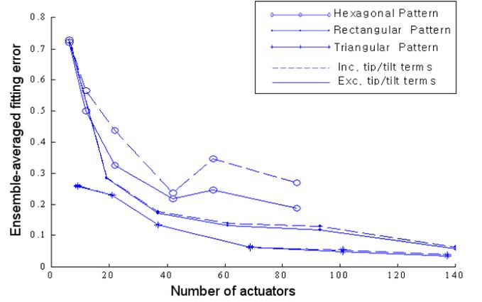
Fig. 6. Ensemble-averaged fitting errors for atmospheric distortion.
