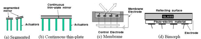
Fig. 1. AO deformable mirrors.
