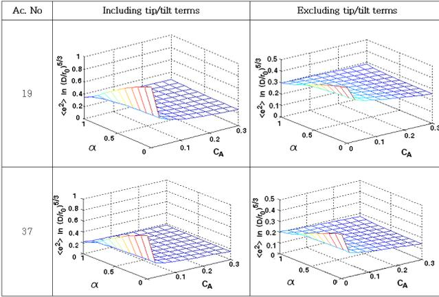
Fig. 5. Ensemble-averaged fitting errors of the triangular layouts (19 and 37 actuators) for atmospheric distortion.
